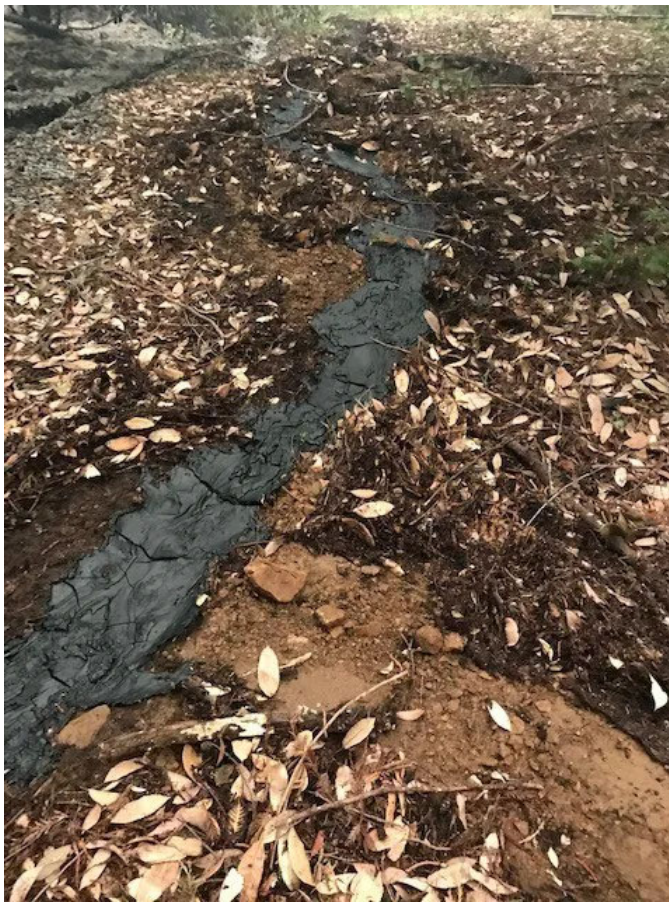
The pipes that melted in Boulder Creek were made of polyethylene — a plastic that can release toxic compounds. (San Lorenzo Valley Water District — Contributed)
